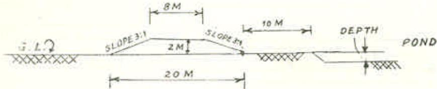
CROSS-SECTION OF SECONDARY DYKE
