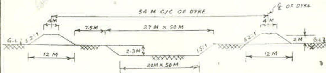
CROSS-SECTION OF SILT TRAP
