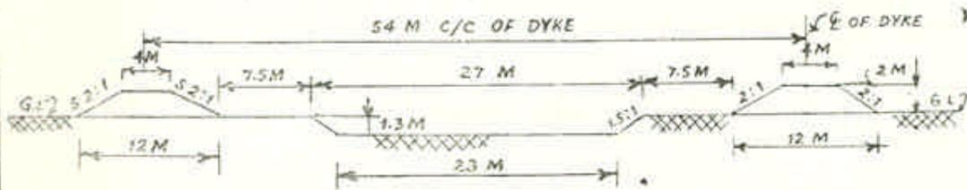
CROSS-SECTION OF FEEDER CANAL AND CANAL DYKES
